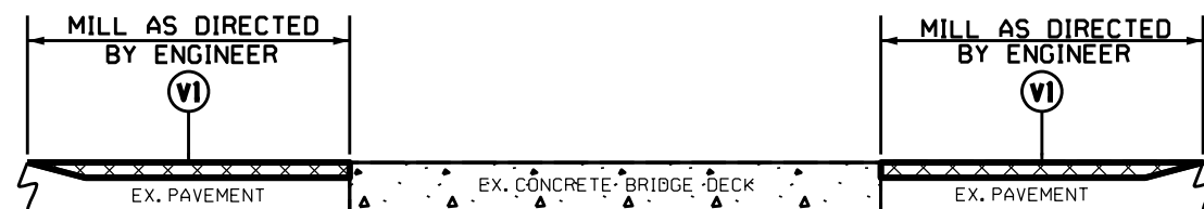
DETAIL 2 BRIDGE MILLING
